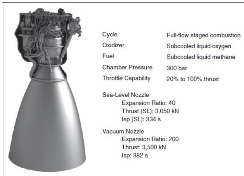
Fig 5. Key characteristics of the Raptor engine [2]
