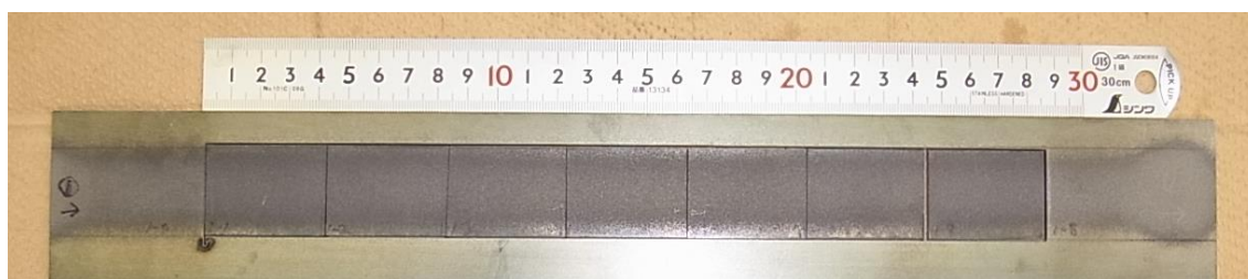
Fig. 5.1. Photograph of SPHC specimen cut by laser after being grit-blasted.
