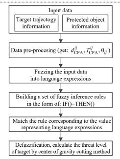
Fig. 4. Fuzzy model diagram to assess the target threat value
