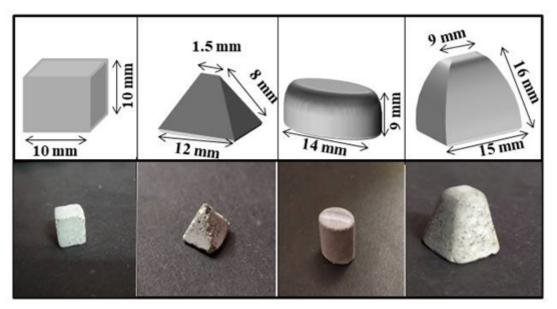
FIGURE 6. Produced Synthetic aggregates in various shape and sizes.
