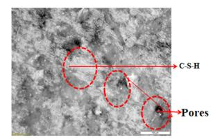
FIGURE 19. Optical Microscopic images of the fracture surface of synthetic aggregates.
