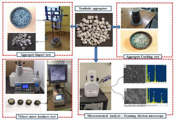
FIGURE 8. Pictorial representation of several tests conducted on produced synthetic aggregates.
