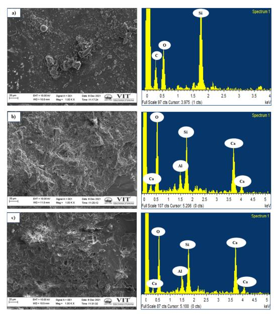
FIGURE 14. Morphological view of (a) Natural aggregates (b) Synthetic aggregates (c). Fiber intruded synthetic aggregates.
