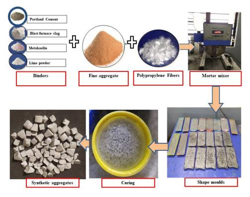
FIGURE 5. Manufacturing process of synthetic aggregates.
