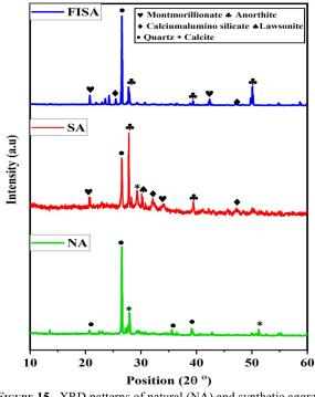
FIGURE 15. XRD patterns of natural (NA) and synthetic aggregates (SA, FISA).
