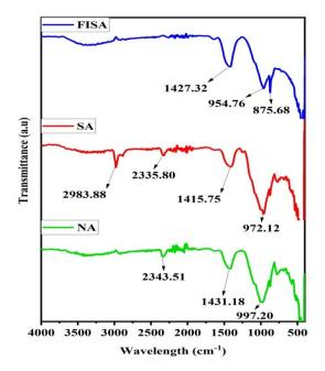
FIGURE 16. FTIR spectrums of natural aggregates and synthetic aggregates.
