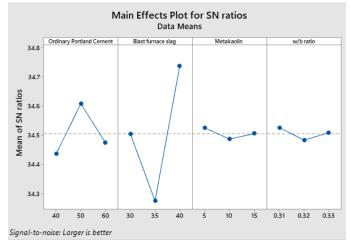
FIGURE 4. Optimized mix proportion by using Taguchi experimental design.
