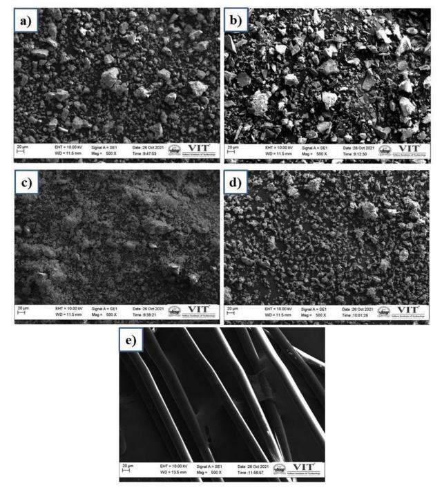
FIGURE 2. Morphological view of (a) OPC (b) GGBFS (c) MK and (d) LP (e) PPF.
