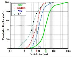
FIGURE 1. Particle size distribution curve of raw binders.
