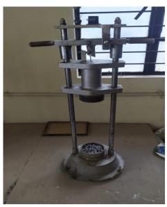
FIGURE 12. Aggregate Impact test apparatus.
