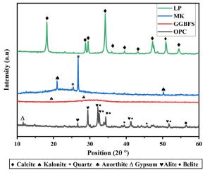
FIGURE 3. XRD patterns of raw binder materials.
