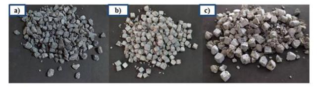
FIGURE 11. Visual appearance after crushing test (a) NA (b) SA (C) FISA.
