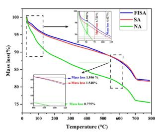
FIGURE 17. TGA curves of (a) natural and synthetic aggregates.
