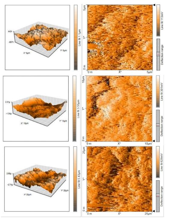
FIGURE 18. 2D and 3D topographical images of NA, SA, and FISA.
