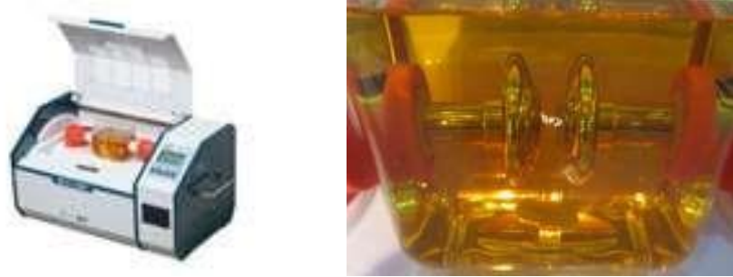
Fig.5 Equipment for testing and Measurement of dielectric strength of oil
