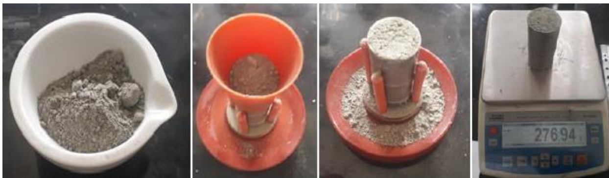
Figure 2. Determination of the bulk density of Amonex.
