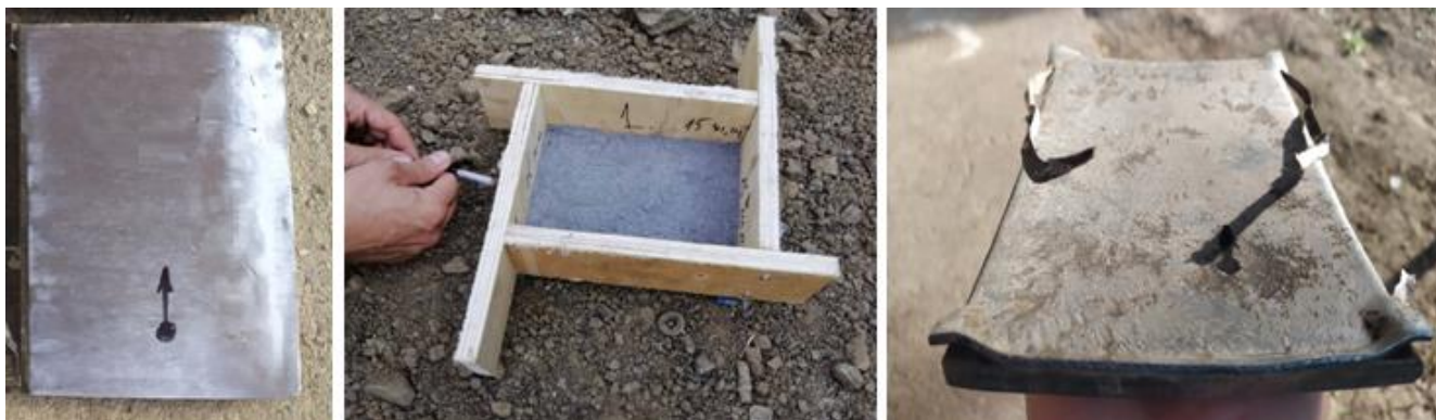
Figure 1. Plate before welding, experimental set-up, and welded plate after the process.
