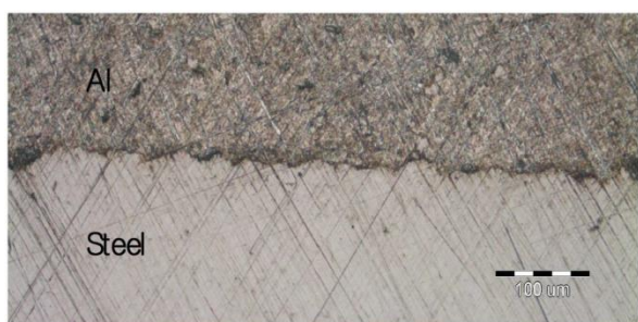
Figure 3. Cross section of the welded material.
