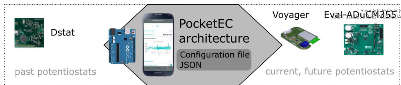
Figure 1. Schematic of the PocketEC app communicating, via Bluetooth, with MCU based potentiostats. We demonstrate communication with established platforms such as the DStat as well as a custom-made Voyager board and the commercially available EvalADuCM355 board. An Arduino board was used to act as buffer between the DStat and the PocketEC app as the latter was designed for real-time communication and the former requires a buffer.
