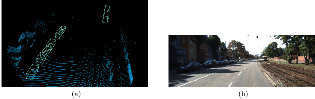
Figure 4.2: Sparse 3D point cloud (a) and its corresponding image (b) from KITTI scene 000045 (aspect ratio and exact sensor position are different). Key to interpret the point cloud: black - empty space; light blue - recorded point; light green - bounding box showing object location.
