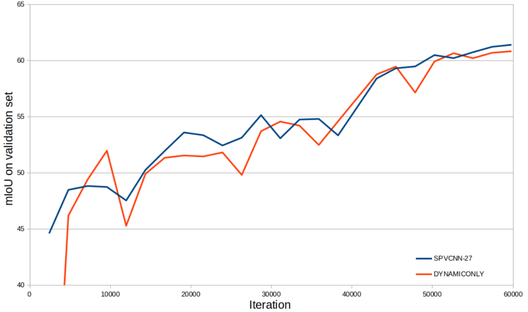
Figure 4.8: Baseline model SPVCNN-27 performs better than a modification that fuses only point of dynamic objects (DYNAMICONLY) and selects its input into feature fusion block based on its own output on previous step.
