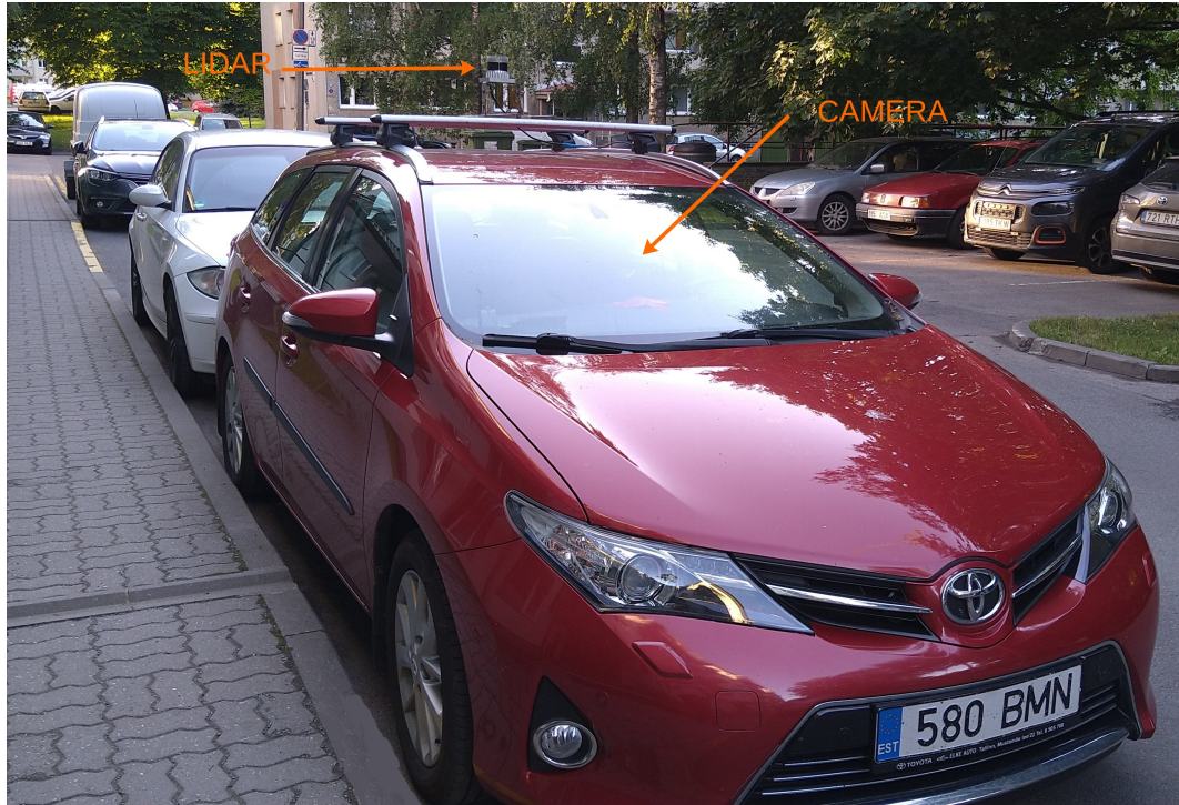
Figure 6.1: Test car system complete with the OS1 lidar and Logitech Brio 4K camera. Locations of the lidar and the camera are indicated by the orange arrows.
