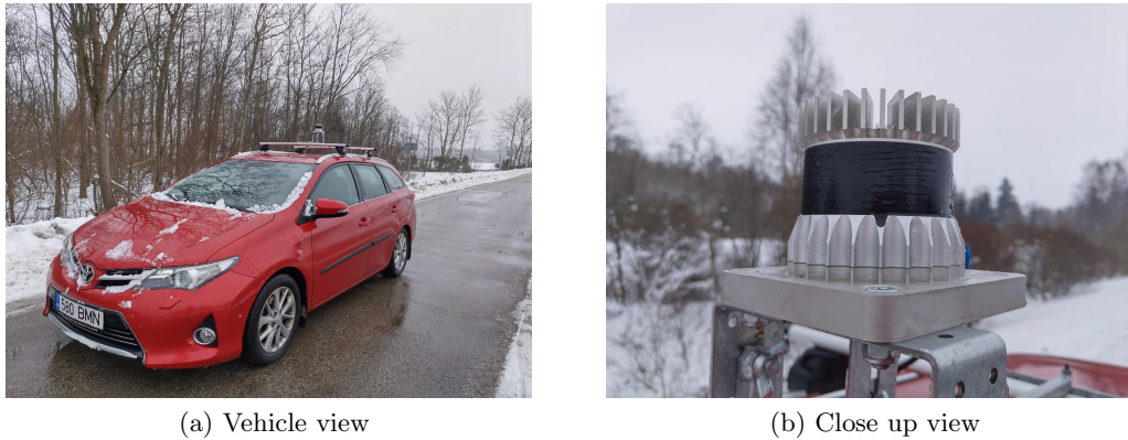
Figure 2.2: Ouster OS-1 lidar mounted on our research vehicle.
