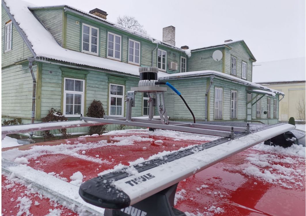
Figure 5.5: A completed mounting rack assembled on top of the test car driving in a historical district in Haapsalu, Estonia. The installation takes into account that the surface of the car might have some snow.
