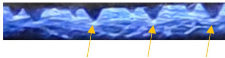
Fig. 5 An optical image of plasma near the pyramid electrode in the pyramid micro DBD reactor to visualize the plasma at a voltage of 6.5 kV. CO 2 flow: 20 ml min -1 . The arrows are pointing at the areas near the tips of pyramids where intense light emission can be seen
