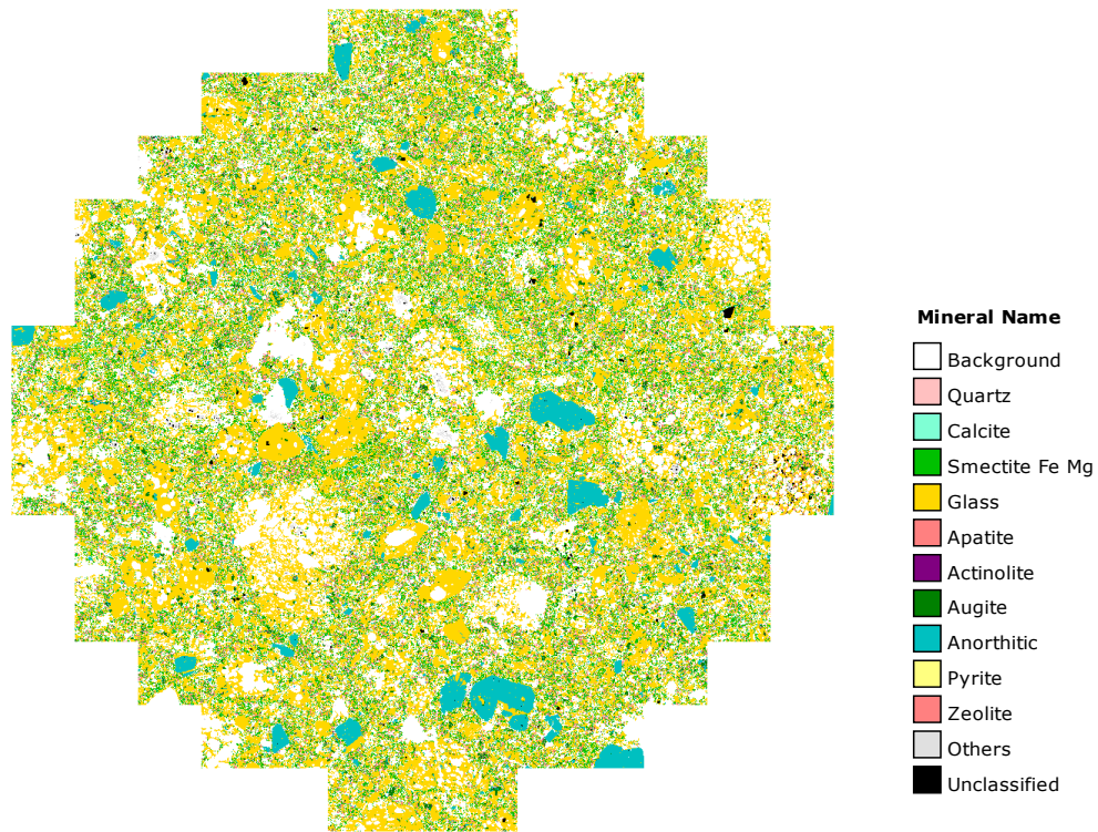
Supplementary Figure A.III-6: Mineral distribution of hyaloclastite, TT to 600 °C for 12 hours, and acquired using QEMSCAN at 20 µm resolution.
