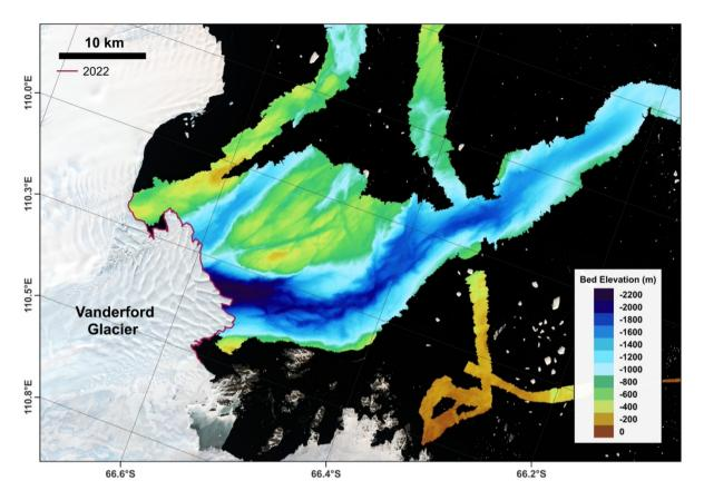
Figure 10. Bathymetry mapped at the front of Vanderford Glacier, collected during RSV *Nuyina's* maidan voyage to Antarctica (Commonwealth of Australia, 2022). Background satellite imagery was collected in February 2022, with red line showing the associated digitised terminus position.
