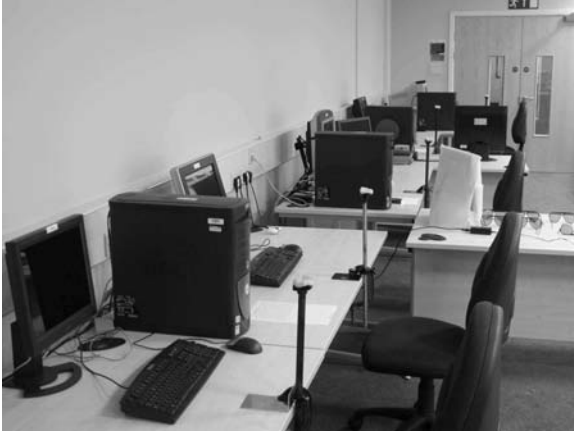
Figure 4. The environment used, where possible displays had chin-rests to guide participants to the ideal viewing position, the displays were placed against a blank background and any reflections of objects or lights behind participants were eliminated.
