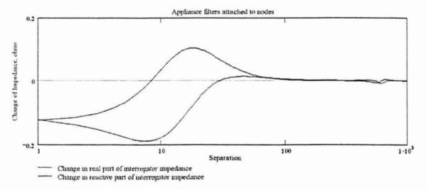
Figure 11: RWD modulation sensitivity versus distance between RWD and RFID tag. Non-zero values on either the red or blue trace indicate potential for receiving data from the tag.
