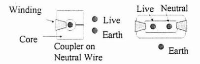
Figure 5: Two possible coupler configurations
