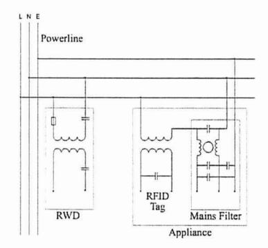
Figure 9: Experimental passive system showing coupling of RFID tag and RWD. Utilisation of a typical appliance mains filter is also shown.
