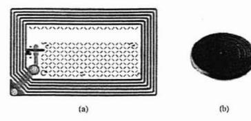
Figure 1: Conventional RFID tags (a) a typical inductive antenna for' label' style tags – the chip is marked red, (b) a packaged 'button' style tag in which the antenna coil and chip are sealed.
