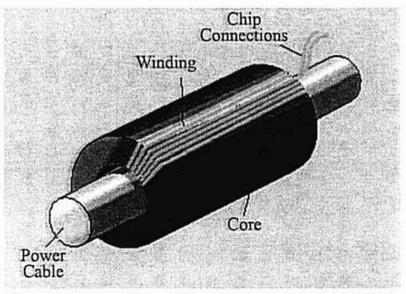
Figure 4: The coupler is simply composed of a copper winding around a ferrite core, to which an RFID chip is attached.
