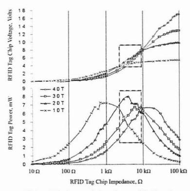
Figure 6: Design graphs showing measured voltage and power available at the coupler as a function of connected load. Boxed regions indicate suitable conditions for transponder chip overation.
