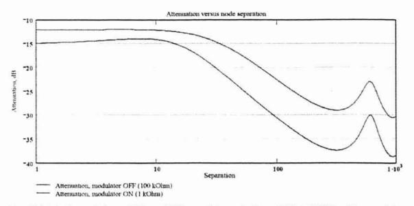
Figure 10: Calculated attenuation between RFID tag and RWD versus their separation distance. Modulator ON/OFF conditions occur during communication.
