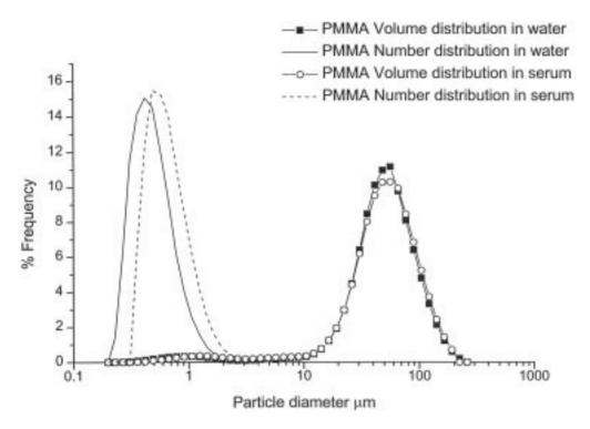
Figure 1 LALLS particle size distribution plots by both number and volume for PMMA powder dispersed within distilled water and digested bovine serum carrying media.
