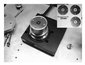
Figure 2. Standard OSCA Lyot mask mounted on a step-motor rotation stage. Other available Lyot masks are shown inset.
