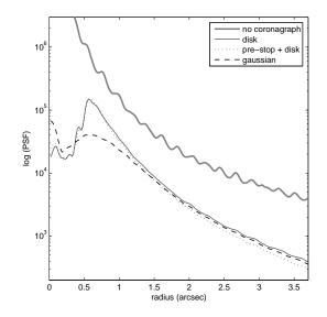
Figure 6. Simulated PSF profiles for the different shaped coronagraphic focal masks, the standard (80,20) Lyot stop was used for each. Characteristic width for each mask is 1.0 arcsec. Phase-screens corrected with a NAOMI-like simulated system - 2000,  $256 \times 256$  phase-screens with an 4 times FFT padding factor. Peak for no-coronagraph lies at  $7 \times 10^8$ .
