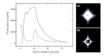
Figure 13. Cross-sections taken in the high-contrast  $(45^{\circ})$  direction from *H*-band images (a) without OSCA (solid line) and (b) with 2.0 arcsec mask (dashed line). The peak at zero is due to the OSCA mask having a small throughput. The jagged drop to zero (< 25 pixels) with no coronagraph is due to detector saturation. The INGRID pixel scale is 0.04 arcsec/pixel.
