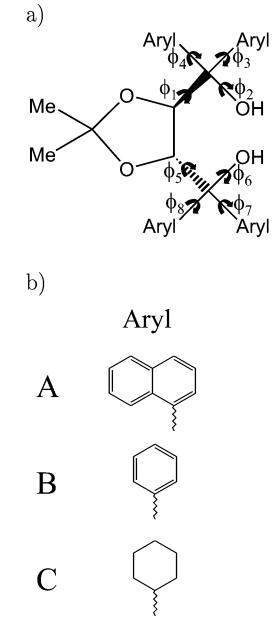
FIG. 3. (a) Basic TADDOL structure showing the flexibility around dihedral angles  $\phi_1 \rightarrow \phi_8$ . (b) TADDOL derivatives A, B, C, where the structures shown are the Aryl substituents in (a).
