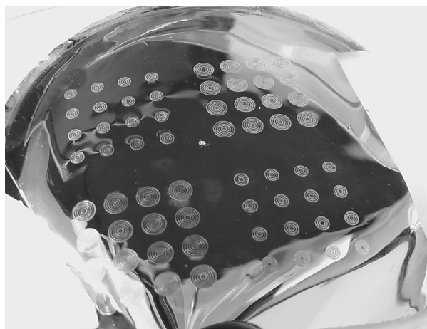
Fig. 6. Fabricated annular devices on a thin and flexible SU8 substrate.
