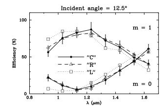
Fig. 4. Diffraction efficiency measured for an incident angle of  $12.5^{\circ}$ . Throughputs measured at the centre are shown by solid circles (and solid line), and those at the other two positions are indicated by open triangle (and dashed line) and open square (and dotted line). The upper three lines are for the m = +1 order diffracted light and the lower ones are for the 0th order light.
