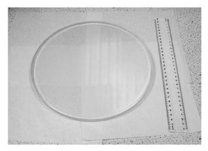
Fig. 1. A picture of the sample VPH grating. The grating has a diameter of 250 mm with a line density of 385 lines/mm.
