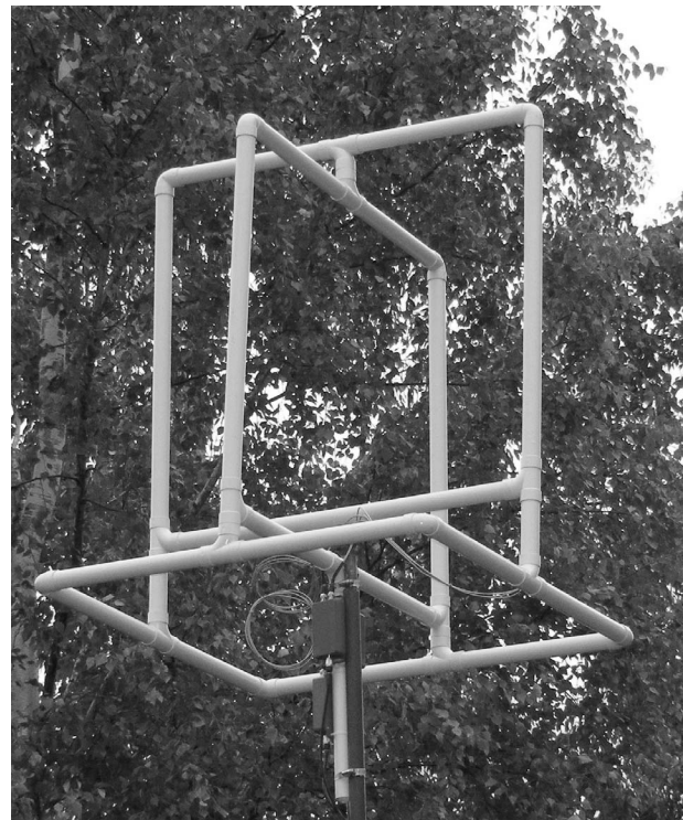
Figure 2. “X-Y-Z” loop array: example of a compact HF receiving antenna array composed of three mutually orthogonal square loop antennas.
