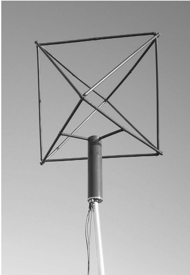
Figure 3. Ground symmetric loop (GSL) array: example of a compact HF receiving antenna array composed of three square loop antennas inclined at angles so that all have the same geometry with respect to the ground.
