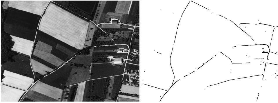
FIGURE 2. Aerial image (© IGN) and result of line network extraction with energy E_0 . Parameter values: [\lambda = 1, \alpha = 0.17, \beta = 0.2, \lambda_i = 2, \alpha_i = 1, \beta_i = 2] .
