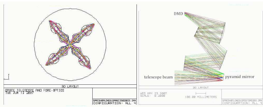
Fig. 8 Fore-optics system. Left: top view (all channels); Right: side view (one channel).
