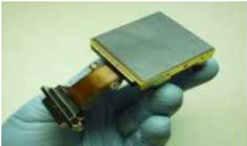
Fig. 11 A 2k×2k buttable Focal Plan Array developed for JWST.
