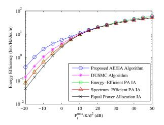
Fig. 10. Energy efficiency comparison of different algorithms in a 3-user IA-based network with 2 antennas at each transceiver. The threshold  $\lambda$  is set to 5%. Energy efficiency is logarithmically scaled.
