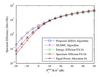
Fig. 8. Spectrum Efficiency comparison of different algorithms in a 3-user IA-based network with 2 antennas at each transceiver. The threshold  $\lambda$  is set to 5%. Spectrum efficiency is logarithmically scaled.
