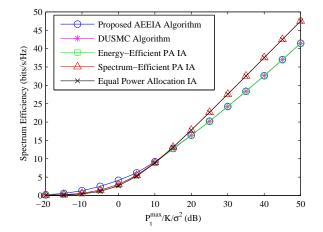
Fig. 7. Spectrum Efficiency comparison of different algorithms in a 3-user IA-based network with 2 antennas at each transceiver. The threshold  $\lambda$  is set to 5%. Spectrum efficiency is linearly scaled.
