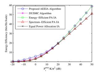
Fig. 9. Energy efficiency comparison of different algorithms in a 3-user IA-based network with 2 antennas at each transceiver. The threshold  $\lambda$  is set to 5%. Energy efficiency is linearly scaled.
