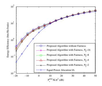
Fig. 14. Energy Efficiency comparison of the proposed AEEIA algorithm with and without fairness, when K = 3.  $N_f$  is equal to 2, 4, 8 and 16, respectively when fairness is considered.
