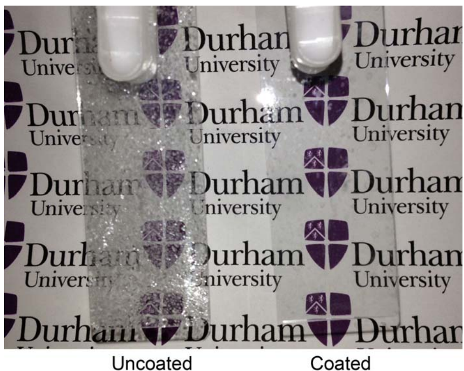
Figure 4: Demonstration of anti-fogging following exposure to water vapour (fogging): on uncoated glass slide and poly(Et- alt -MA)–fluorosurfactant complex solvent cast from dimethylformamide. Similar behaviour was observed for poly(St- alt -MA)–fluorosurfactant and poly(St- co -MA)–fluorosurfactant complex dip coated glass slides using dimethylformamide solvent.
