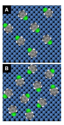
Figure 3. Schematic representation of plausible ClBz structures. Molecules have been represented by their vdW radii. **A**: rectangular phase. **B:** hexagonal phase. Color code: green (chlorine), gray (carbon), white (hydrogen) and blue (silver).
