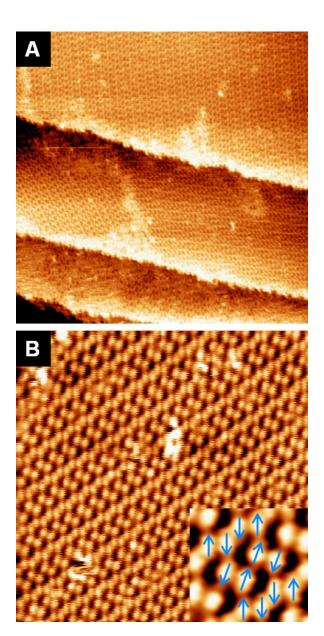
Figure 5. Phenylacetylene island growth on Ag(100). See text. Exposure: 4L. A: (75 nm x 75 nm) I=0.31 nA V=1.89 V. B: (25 nm x 25 nm) I=0.40 nA V=2.31 V. Inset: Magnified image with a superimposed dipole model illustrated as blue arrows.
