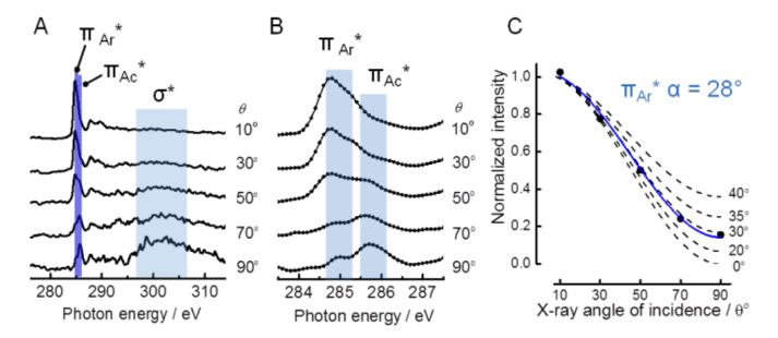
Figure 6. **A:** C K-edge NEXAFS spectra acquired at five angles of photon incidence  $\theta$  for a ~ 1.0 ML coverage of PA on Ag(100) at 170 K. **B:** Leading  $\pi^*$  resonances, expanded scale (Ar = aromatic; Ac = Acetylenic). **C:** Curve fitting analysis of q dependence of  $\pi^*$  resonance **A** to estimate the phenyl ring tilt angle,  $\alpha$ .
