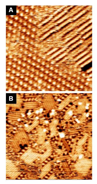
Figure 4. STM images showing progressive formation of biphenyl with increasing temperature. **A**: 25.0 nm x 25.0 nm) I=0.44 nA V=2.1V, following further annealing (Si diode temperature = 240 K). **B**: 25.0 nm x 25.0 nm, I=0.38 nA V=2.1 V following annealing to higher temperature (Si diode temperature = 295 K).
