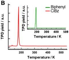
Figure 8. TPD and TPR spectra for both reactants. **A:** TPD spectrum of PA adsorption on clean Ag(100) at 105 K Exposure: 0.6 L. Inset: TPR spectrum of the reaction product DPDA. Exposure: 15L. **B:** TPD spectrum of ClBz adsorbed on clean Ag(100) surface at 105 K. Exposure: 0.2 L. Inset: TPR spectrum of the reaction product BP. Exposure: 6 L. All spectra were filtered to reduce noise signal.
