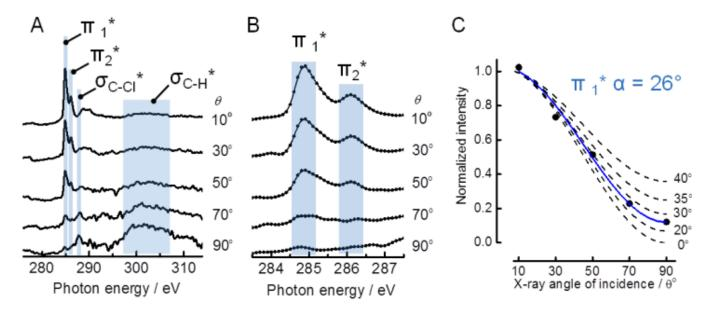
Figure 7. A: C K-edge NEXAFS spectra acquired at five photon incidence angles  $\theta$  for a ~ 1.0 ML coverage of ClBz on Ag(100). **B**: Principal  $\pi^*$  resonances expanded scale. C: Curve-fitting analysis of the photon angle dependence of  $\pi_1^*$  resonance to estimate the corresponding phenyl ring tilt angle,  $\alpha$ .
