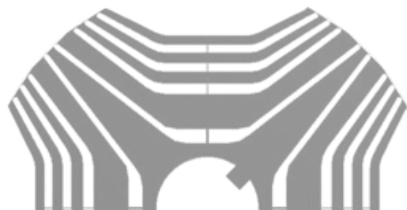
Fig.7. Optimized rotor geometry showing flux guides and q-axis cutouts.
