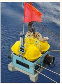
**5** An ocean-bottom seismograph (OBS) being launched on JC132. The yellow section contains spherical glass floats; the sensors and data logger are in the box below. The concrete anchor is released on command from the ship to return the instrument to the surface.
