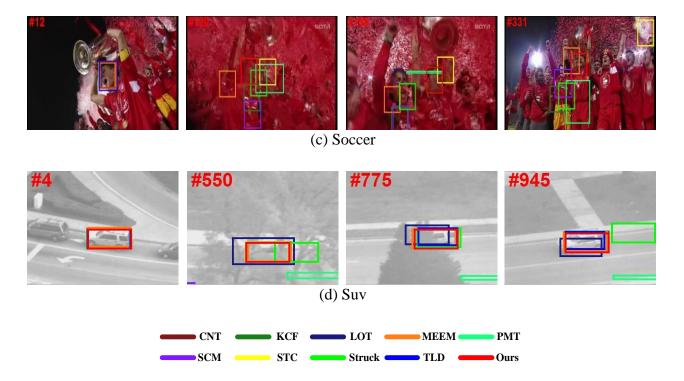
Fig. 8 Screen shots of tracking results under the situations of heavy occlusion.
