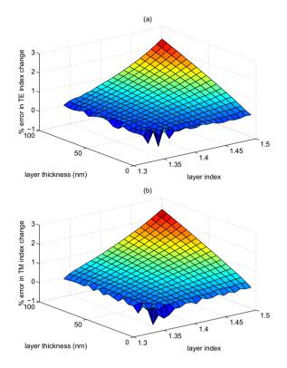
Figure 3. The percentage error in the calculated change of (a) the TE mode index and (b) the TM mode index shown in figure 2 relative to the change obtained using a full numerical method.
