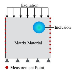
Figure 1: Schematic for the numerically simulated examples representing characterization of an elastic modulus distribution with an inclusion based on mechanical testing involving the excitation and measurement points shown.
