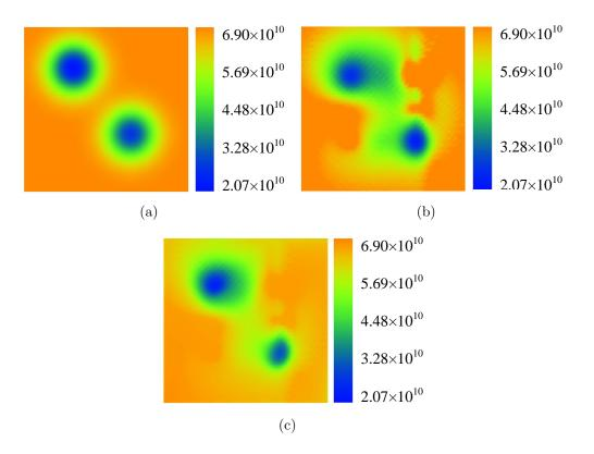
Figure 5: Representative two circular inclusion example of (a) the target elastic modulus distribution, (b) the elastic modulus distribution estimated with the direct inversion approach with Gappy POD full-field displacement reconstruction, and (c) the elastic modulus distribution estimated with gradient-based optimization initialized with the direct inversion solution for the simulated aluminum plate example (color contours in units of Pa).
