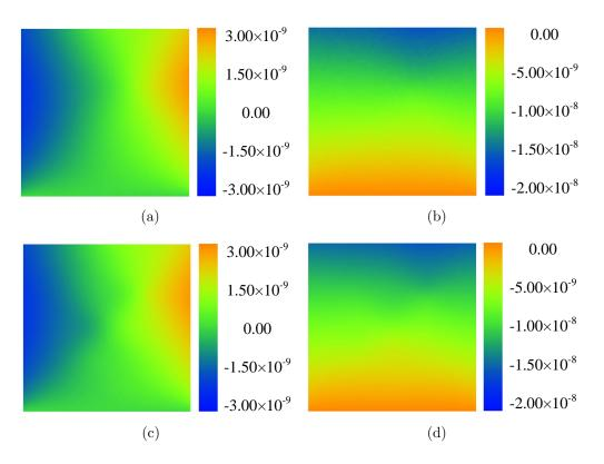
Figure 3: Representative single circular inclusion example of the (a) horizontal and (b) vertical components of a simulated experimental displacement field with 1% Gaussian white noise and the (c) horizontal and (d) vertical components of the corresponding reconstructed full-field displacement from Gappy POD with the partial-field measurements for the simulated aluminum plate example (color contours are in units of m).
