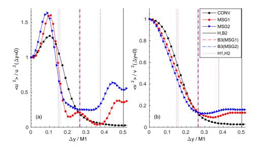
FIG. 10. The spanwise distribution of normal stresses at their peak locations behind the thickest bar B1 ( $\Delta y = 0$ ). The distribution is symmetric about  $\Delta y = 0$  and 0.5M (H or B2). The characteristic line positions are also marked.
