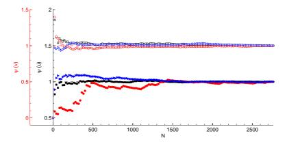
FIG. 2. Convergence history for the two fluctuating velocity components  $\psi(u)$  and  $\psi(v)$ . Data sampled at the location of the strongest fluctuations behind the thickest bar B1. The data are normalised by their final values.  $\blacksquare$ : CONV;  $\bullet$ : MSG1;  $\triangleright$ : MSG2. Filled symbols for the u component and open symbols for v. Only every twentieth data point are shown.
