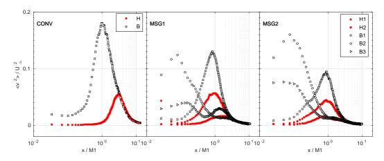
FIG. 9. The normalised spanwise component of Reynolds stress  $\langle v^2 \rangle / U_{\infty}^2$  along the characteristic symmetry lines.
