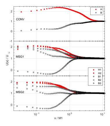
FIG. 7. The streamwise development of the mean streamwise velocity U(x) behind H and B.
