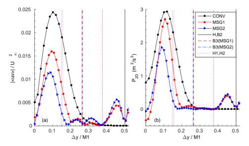
FIG. 13. Spanwise distribution of Reynolds shear stress  $\langle uv \rangle$  and  $\mathcal{P}_{2D}$  at the peak  $\mathcal{P}_{2D}$  locations behind the thickest bar B1 ( $\Delta y = 0$ ). (a) the magnitude of  $\langle uv \rangle$  normalised by  $U_{\infty}^2$ , in order to make direct comparison with figure 8 and 9; (b) the absolute value of  $\mathcal{P}_{2D}$ . The distributions are symmetric about  $\Delta y/M_1 = 0$  and 0.5.
