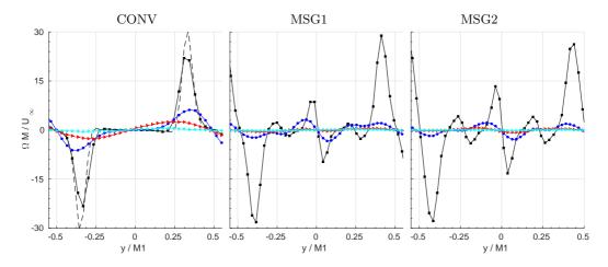
FIG. 6. Spanwise distribution of the in-plane vorticity  $\Omega_z$  at locations  $x/M_1=0.13,\ 1.2,\ 2.5$  and 5.0. Line definitions as in figure 5.
