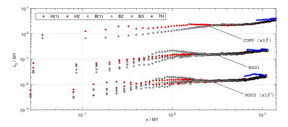
FIG. 15. The streamwise development of the integral length scale  $L_f$  defined by equation 5, with  $\mathbf{x}_0$  on all the characteristic symmetry lines. The  $L_f$  of CONV and MSG2 are shifted up and down one decade as indicated. Only every fourth data points are plotted.
