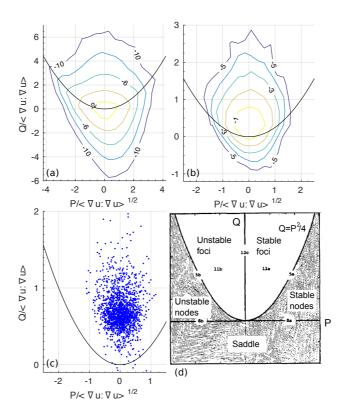
FIG. 17. The joint PDF of P and Q at x=300 mm ( $x=8M_1$ ) downstream of the CONV grid. (a) Every  $\omega_z$  data point is included; (b) the peak  $\omega_z$  data points only. Contour levels in (a) and (b) are log scaled. (c) the scatter plot of the highest 10% population of the peak  $\omega_z$  in (b). The plots for MSG1 and MSG2 show similar patterns. (d) Classification of critical points on the P-Q chart; see Perry & Chong<sup>28</sup> or Chong et al.<sup>8</sup> for details.
