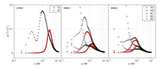
FIG. 8. Development of the normalised streamwise component of Reynolds stress  $\langle u^2 \rangle/U_\infty^2$  along the characteristic symmetry lines.
