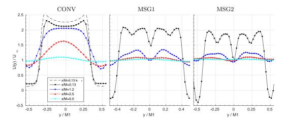
FIG. 5. The spanwise distribution of the mean streamwise velocity component U(y) at downstream locations  $x/M_1=0.13,\ 1.2,\ 2.5$  and 5.0. U(y) is normalised by the free stream velocity  $U_\infty$ . Only about one period of the spanwise range is presented, from one B1 to the next B1. RANS predictions using the  $k-\epsilon$  model is included for CONV at  $x/M_1=0.13$  (dashed line) for comparison.
