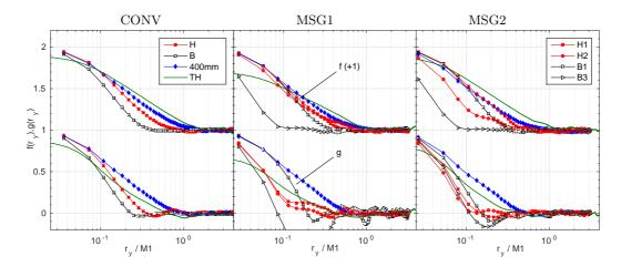
FIG. 14. The longitudinal and normal correlation functions  $f(r_y)$  and  $g(r_y)$  at the maximum stress location along characteristic symmetry lines, as well as at x = 400mm. f and g based on the Taylor hypothesis (denoted TH) are also shown. f is shifted one unit upwards. Functions behind B2 are not presented since peaks are not clearly identified there.
