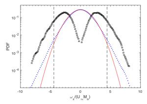
FIG. 16. The PDF of the fluctuating vorticity  $\omega_z$  measured at  $x=300 \mathrm{mm}$  downstream of the CONV grid. Line ···· denotes the PDF of all the data point. –, is a Gaussian best fit;  $\Box$ , the PDF of the peak  $\omega_z$ ; — indicates the minimum  $\omega_z$  value of the highest 10% population group of the peak  $\omega_z$ . The plots for MSG1 and MSG2 show similar patterns.
