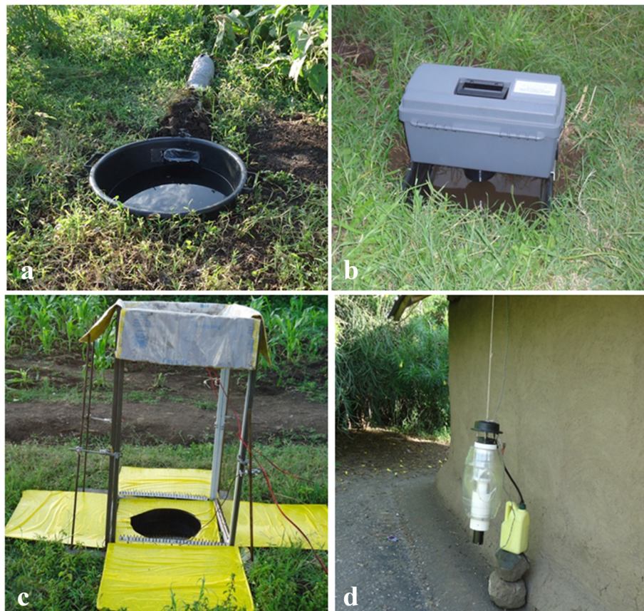
Fig. 5 Traps set up for comparison under field conditions in Kombe village, western Kenya. a The OviART gravid trap. b The Box gravid trap. c Square of electrocuting nets around pond with yellow sticky boards to preserve electrocuted mosquitoes. d the MM-X trap fixed on outside of house
