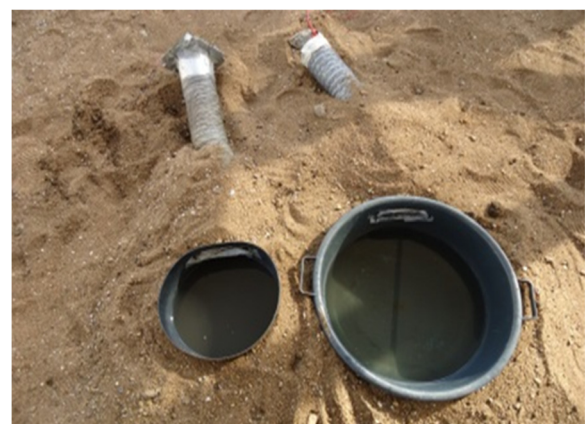
Fig. 3 Comparison of the prototype OviART gravid trap with small basin (left) and improved trap with a basin twice the size of the prototype (right)
