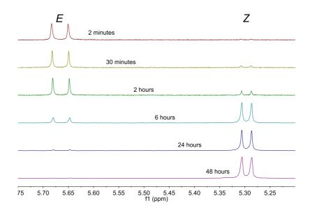
**Figure 3.** The <sup>1</sup>H NMR spectrum of **3a** in chloroform- $d_1$  monitored over 48 hours after a D<sub>2</sub>O shake experiment. The  $\alpha$ -carbonyl proton of the *Z*- and *E*-isomers are shown. Immediately after agitation with D<sub>2</sub>O the *E*-isomer predominates (2 mins), but over time is found to preferentially isomerize to the thermodynamically favored *Z*-isomer.
