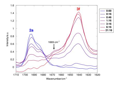
Figure 1. The *in situ* FTIR spectra of the reaction between 1f and 2a at selected time points (time proceeds from blue to red). The decline of the carbonyl stretch of 2a (1693 cm<sup>-1</sup>) and the consequent rise of the carbonyl stretch of 3f (1640 cm<sup>-1</sup>) is shown as the reaction proceeded. The carbonyl stretch of 2a fell to 50% intensity after approximately 2 minutes. A subtle shoulder is evident at 1669 cm<sup>-1</sup> that corresponds to the *E*-isomer of 3f.
