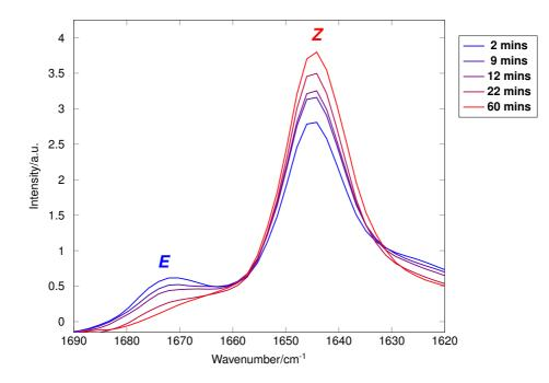
**Figure 5.** *In situ* FTIR monitoring of the 1620-1690 cm<sup>-1</sup> region of **3a** in chloroform- $d_1$  immediately after isolation. The relaxation of the *Z/E* equilibrium was followed by monitoring the intensity of the carbonyl stretches of the *E*- and *Z*-isomers over time (time proceeds from blue to red). Initially a small amount of the *E*-isomer (1672 cm<sup>-1</sup>) is present, but this converts to the *Z*-isomer (1644 cm<sup>-1</sup>) over 1 hour.<sup>22</sup>
