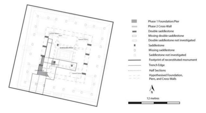
Figure 5: Plan of Trench at Kasthmandap.
