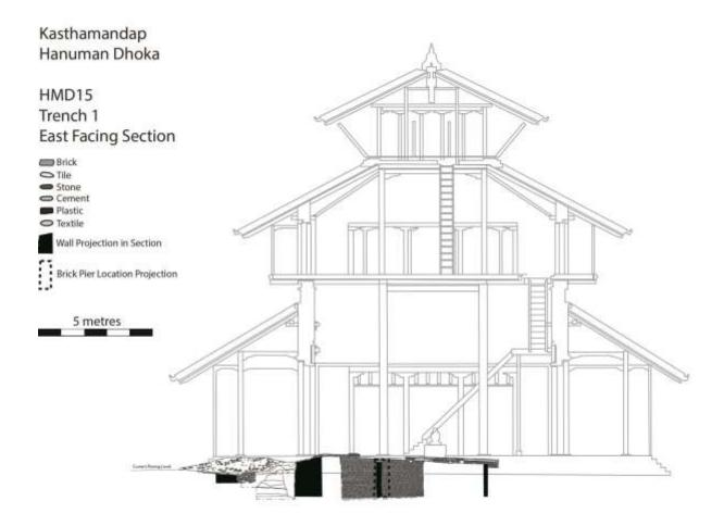
Figure 27: East facing section of Trench, illustrating depth of foundations, with superimposed elevation of the Kasthamandap before collapse (Elevation of Kasthamandap, after Korn 2007).
