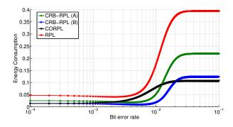
Fig. 8. Average energy consumption for a single hop operation against bit error rate (10, 000 packets are transmitted, and node density =  $3 \times 10^{-4}$  nodes per unit).
