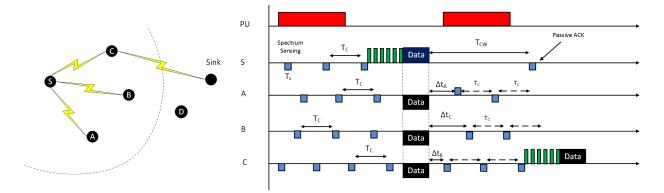
Fig. 3. Timeline of CRB-RPL routing with an illustrated scenario of sender and receiver nodes
