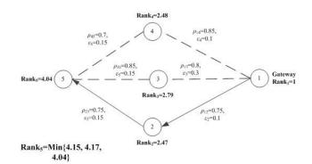
Fig. 2. Rank computation based on CTQ. The rank of a node is depended on link quality and fractional area between client nodes and PU transmitters. The lowest rank computed based on different parent nodes is adopted.
