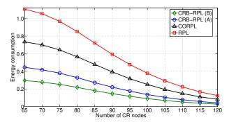
Fig. 9. Average energy consumption (Joule) for a single hop operation against node density (10, 000 packets are transmitted).
