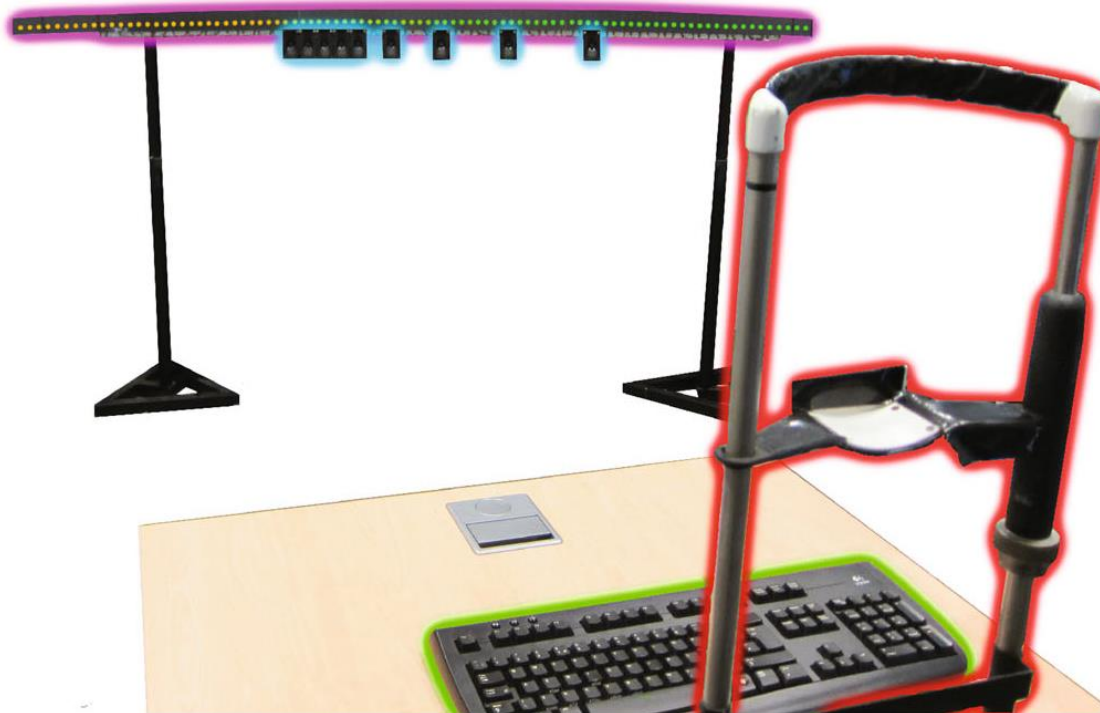
Figure 1: The Ring of LEDs and Speakers. On each presentation a flash of lights from a subset of LEDs (outlined in purple) and/or a noise from a speaker (outlined in blue) was presented. Participants maintained their head position fixed at straight ahead, using a chin rest (outlined in red), and entered responses using the keyboard (outlined in green).
