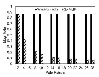
Fig. 5. Winding factors of the 6-slot 4-cSynRM
