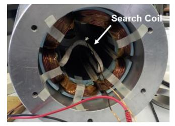
Fig. 8. Removed rotor testing of the prototype machine.
