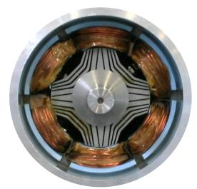
Fig. 1 Single-tooth coil synchronous reluctance motor (6 slot 4 pole).
