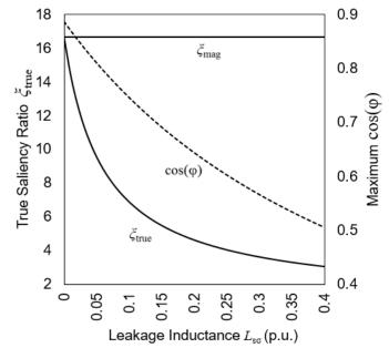
Fig. 4 True saliency ratio  $\xi_{true}$  and maximum power factor capability as a function of per-unit stator leakage inductance with  $\xi_{mag} = 16$ .
