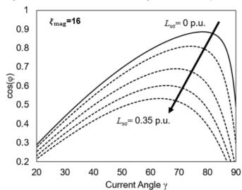
Fig. 3 Power factor curves as a function of current angle for  $\xi_{mag} = 16$  and increasing stator leakage inductance.
