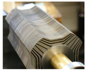
Fig. 6. The prototype rotor showing lamination profile.
