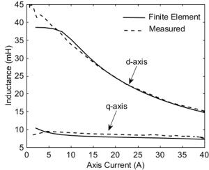
Fig. 7. FEA and measured direct- & quadrature-axis inductances [4]
