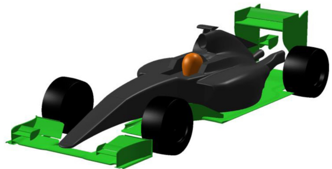
Figure 1. 2014 generic F1 car CAD with key downforce generating surfaces coloured green
