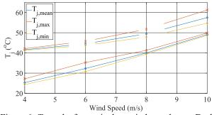
Figure 6: *T<sub>j</sub>* results for equivalent wind speed tests. Dashed lines are simulated results and solid lines and experimental results.
