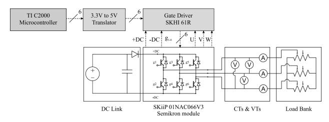
Figure 3: Electrical circuit diagram of the experimental rig.
