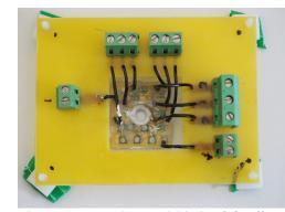
Figure 4: SEMIKRON 01NAC066V3 MiniSKiiP module modified for testing.
