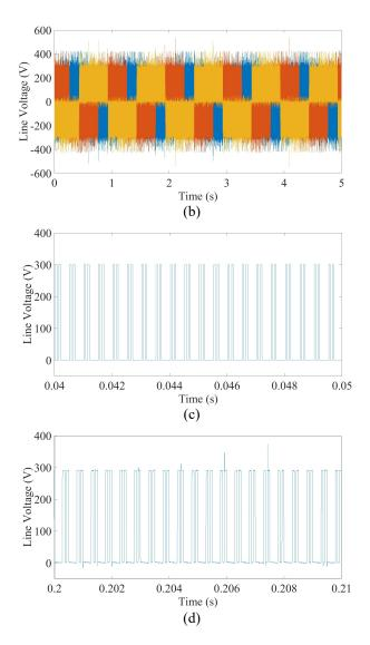
Figure 5: Verification of 3-phase voltage output: (a) simulated voltage, (b) measured voltage, (c) zoomed-in simulated voltage, (d) zoomed-in experimental voltage.
