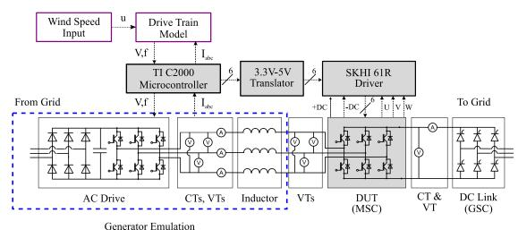
Figure 7: Test bench to allow variable wind condition testing.
