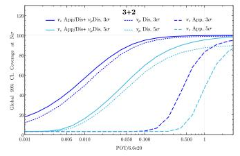
FIG. 11. The same as Fig. 10 but for the 3 + 2 light sterile neutrino scenario. The percentage of 99% CL globally allowed 3 + 2 parameter space that SBN can exclude at the  $5\sigma$  (light blue) and  $3\sigma$  (dark blue) CL for  $\nu_e$  appearance only (dotted),  $\nu_{\mu}$  disappearance only (dashed) and a combined appearance and disappearance fit (solid), as a function of POT.
