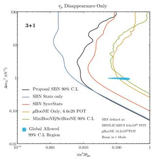
FIG. 7. The estimated 90% CL contours for the combined SBN using  $\nu_{\mu}$  disappearance only. The globally allowed region in  $\Delta m_{41}^2$  and  $\sin^2 2\theta_{\mu\mu}$  is completely covered. Shown also is the prediction for MicroBooNE after 6.6e20 POT.
