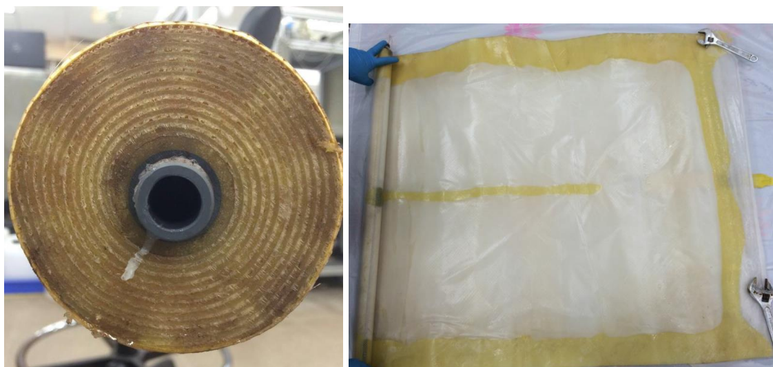
Figure 1 Cross-sectional view of the spiral wound CTA membrane taken out of its module casing (left) and unwound (right)
