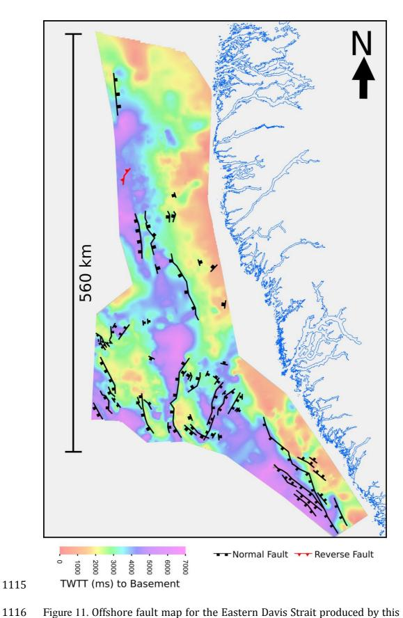
Figure 11. Offshore fault map for the Eastern Davis Strait produced by this study overlain on the basement horizon in TWTT (ms).
