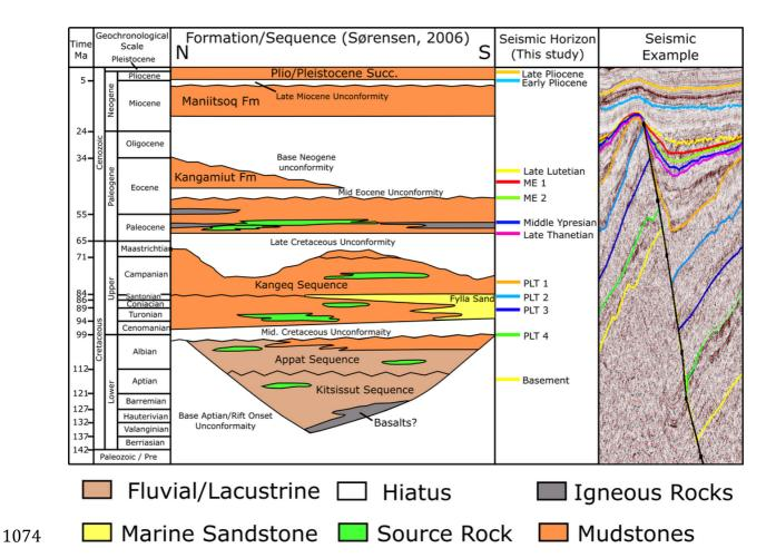
Figure 3. Stratigraphic framework for the study area (Fig. 1) modified from Sørensen (2006) to include the stratigraphic locations of the horizons interpreted in this study and an example seismic section.
