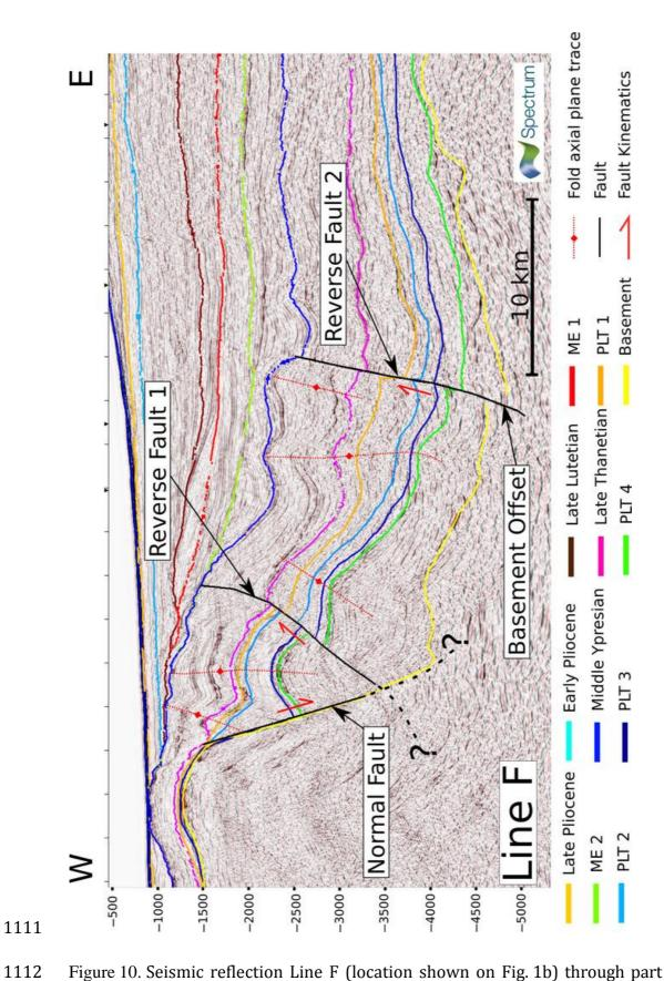
Figure 10. Seismic reflection Line F (location shown on Fig. 1b) through part of the Ikermiut Fault Zone and associated folding predating the Middle Ypresian horizon.
