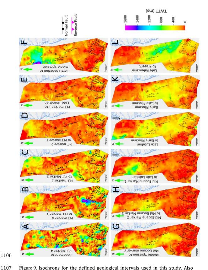
Figure 9. Isochrons for the defined geological intervals used in this study. Also shown are the interpreted faults with transparency increasing through time to indicate the diminishing role of such structures.
