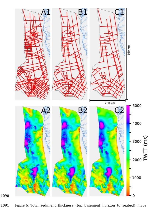
Figure 6. Total sediment thickness (top basement horizon to seabed) maps produced after thinning the seismic grid. The seismic grid above each isochron depicts the lines used to produce the isochron below.
