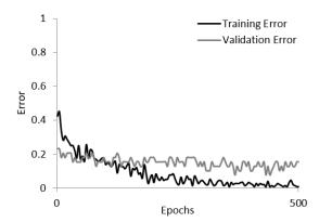
Fig 6. The graph shows the error loss (inverse of AoC) of PodNet on training and validation data subsets for subject 29 data over 500 epochs.
