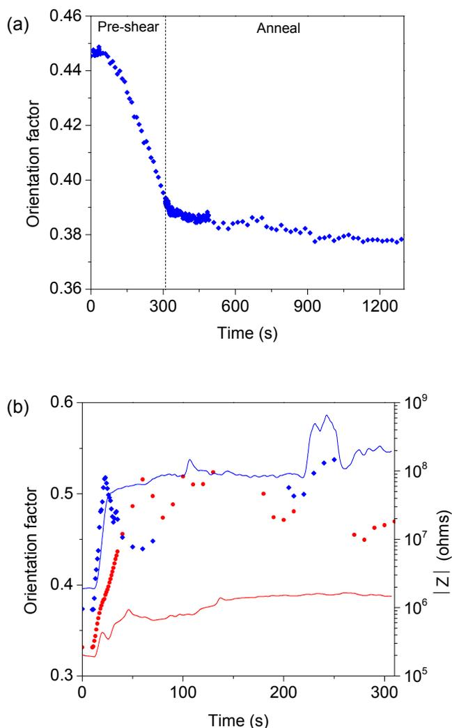
Figure 7. Orientation factors calculated for composites of polystyrene + 5 vol. % GNPs from SAXS under shear at 200 °C. (a) Orientation factor of GNPs during a pre-shear at a rate of  $0.01 \text{ s}^{-1}$  and subsequent annealing step. (b) Orientation factors (symbols) and impedance  $|Z|$  (lines) during shear at rates of  $0.3$  (●—) and  $1.8 \text{ s}^{-1}$  (◆—).
