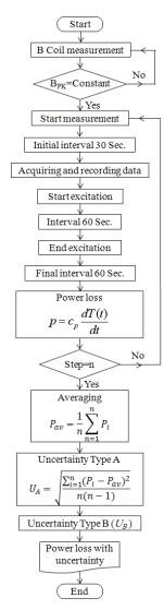
Fig. 3 Flowchart of the measurement system
