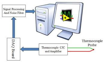
Fig. 2 Basic block diagram of the measuring system
