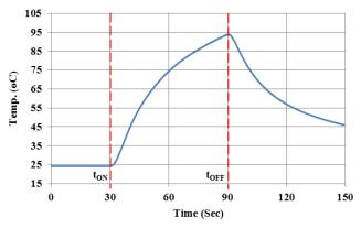
Fig. 19 Temperature rise vs. time at 1.8 T, 50 Hz at point 1 of Fig. 18
