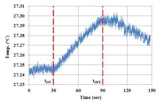
Fig. 16 Temperature rise vs. time at 1.3 T, 50 Hz at point 3 of Fig. 15
