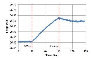
Fig. 10 Temperature rise vs. time due to heating effect at point 1 of a 5 A DC current passing along the copper strip
