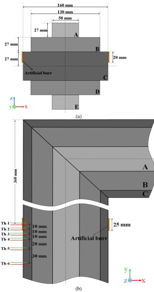
Fig. 18 (a) Cross section of the core and position of the artificial burr (b) Top view of the core and position of the thermocouples
