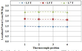
Fig. 14 Localised power loss vs. thermocouple position of NO electrical steel at different flux density
