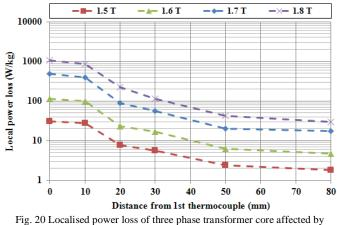
artificial burr versus position of the thermocouples
