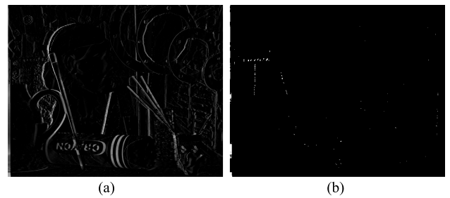
FIGURE 3. The differential map depicts pixel errors of Fig. 2(b) against Fig. 2(a), and the JND map calculated with Eq. (2) contains high intensity pixels denoting noticeable distortions. (a) Differential map. (b) JND map.
