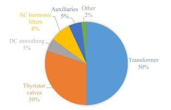
Fig. 8. Evaluation of the heat losses per component of a HVDC station [35].
