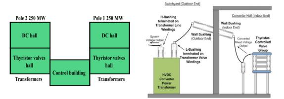
Fig. 18. Vertical (left) and lateral (right) view of transformer and thyristor valve hall of HVDC converter station, adapted from [33,65,66].
