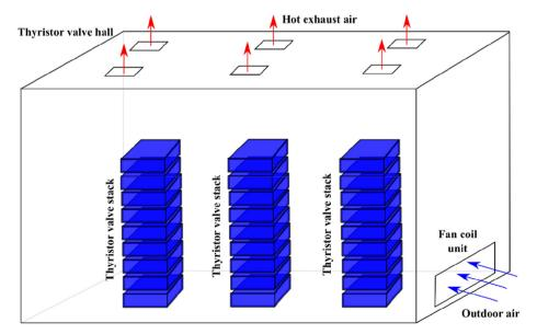
Fig. 9. Ventilation air system of thyristor valves hall.
