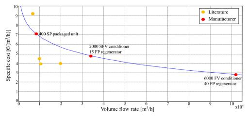
Fig. 21. Specific cost per air volume flow rate of Kathabar LD system.
