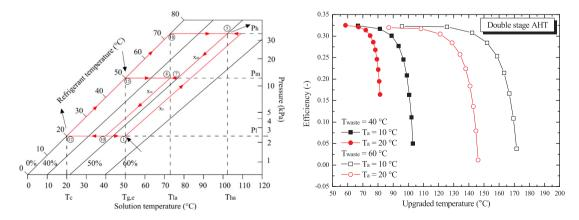
Fig. 15. P-T diagram of double effect absorption heat transformer (left) and achievable temperature lift (right).
