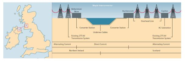
Fig. 7. Schematic diagram of Scotland – Northern Ireland HVDC station [33].
