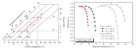
Fig. 14. P-T diagram of single effect absorption heat transformer (left) and achievable temperature lift (right).
