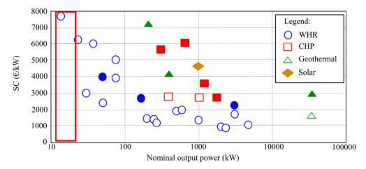
Fig. 20. Specific cost function depending on nominal output power of ORC system, adapted from [68]
