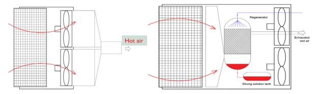
Fig. 16. Air as waste heat recovery medium, used at the downstream (left) and at the upstream of the fan (right).
