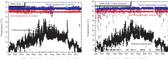
Fig. 12. Ambient air, inlet and outlet cooling water temperature for Pole 1 and Pole 2 in 2009.
