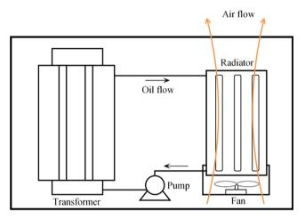
Fig. 11. Schematic diagram of OFAF transformer.
