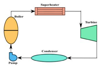
Fig. 6. Schematic diagram of ORC system.
