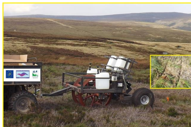
Figure 12. Prototype planting machine for BeadaGel™ being trialled by the MoorLife 2020 project (National Trust and Moors for the Future Partnership). Inset photo: grooves cut into surface vegetation to ensure that Sphagnum gel contacts the peat surface.
