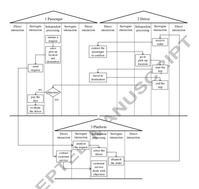
Fig. 3. PCN diagram of online car-hailing service
