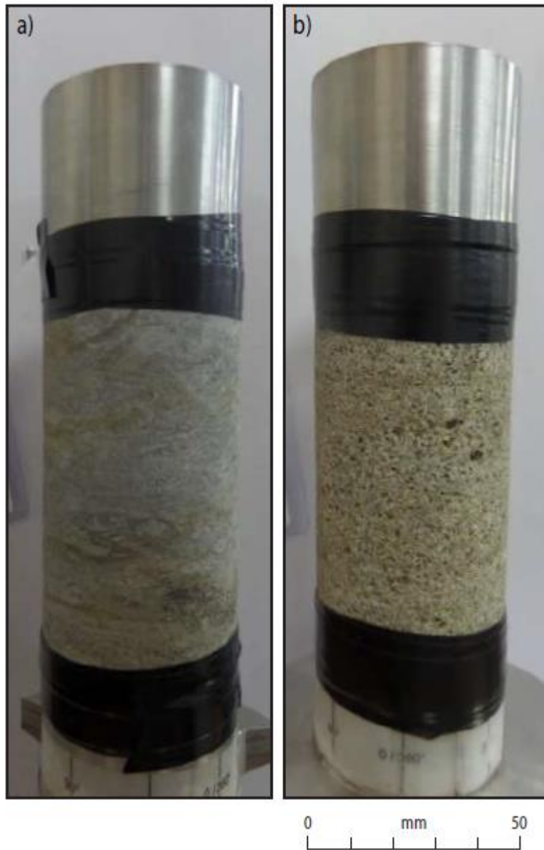
Figure 1. a) Example siltstone sample core. b) Example sandstone sample core. Both cores are 96 mm high, and 48 mm in diameter.
