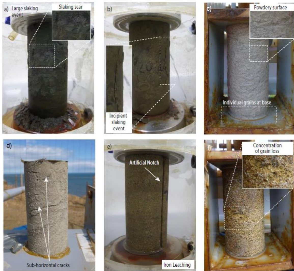
Figure 7. Photographs of weathered samples taken during monitoring experiments. a) Siltstone sample displaying slaking, with detached fragments evident around the base of the container. b) Siltstone core displaying an incipient slaking event characterised by a vertical shallow crack with a narrow aperture. c) Siltstone sample with a 'powdery' surface to touch, with many individual grains at the base of the core. d) Siltstone sample with multiple sub-horizontal cracks at the top and mid-point of the core. e) A sandstone sample with modified geometry ( G ) displaying iron leaching. f) Sandstone sample displaying an area of concentrated grain loss. a), b), and e) were
