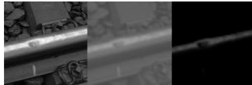
Figure12. From left to right – the input image and the subgraphs from the 133 rd channel of Con1 and ReLU1 produced by the FT-AlexNet for an example squat defect image.
